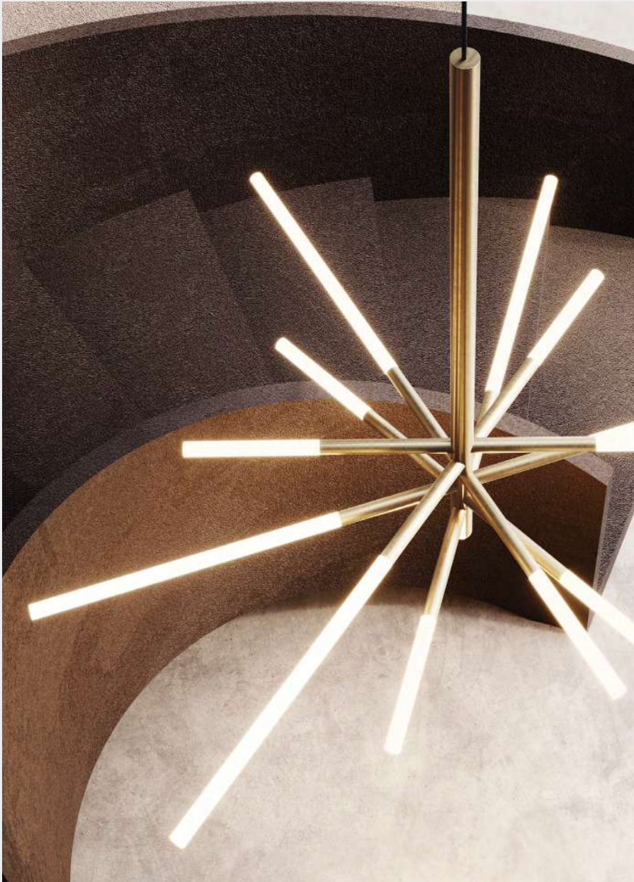
The lamp consists of modules that connect wirelessly through contact points. Each module contains two printed circuits that transfer electricity to the others, illuminating the lamp. The tubular light sources, available in three sizes, are custom-made by Contardi with an E14 24V fitting.
