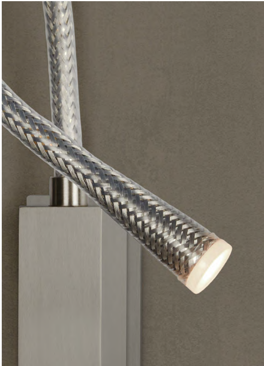
Flexible arm made of brass 0.4" diameter: this prevents from any squeaking even after a prolonged use of the product. In the steel version, the steel mesh covering the tube is protected by a transparent heat-shrinkable silicone sheath.
